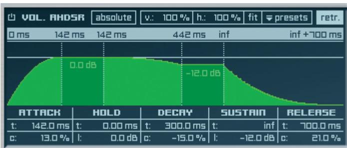
With the VOL. AHDSR curve you can adjust the time flow and simultaneously the volume flow of your Layer, Section or Alternate.
