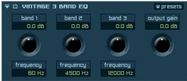
As the name implies: A precise reproduction of a Vintage EQ. The slope of the curve is already determined for each filter.
