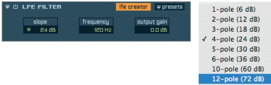
If you are working in a surround format that contains a LFE, you can use this filter to cut high frequencies depending on the selected slope.
