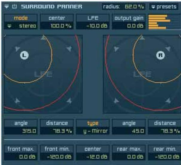
The surround panner enables you to use instruments that contain stereo, mono and surround audio files in any Independence surround environment. Corresponding to the position of the stereo (L & R) or mono (M) or surround (S) icons new volume settings get calculated for all existing channels of your currently selected surround format.
