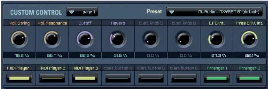
There is a „custom learn“ option for any Independence parameter, so you just have to select this option for the parameter you want to assign to one of the custom control knobs or buttons (in the example we chose the “resonance” parameter of the insert “Multimode Filter” on the “Modules” page):
