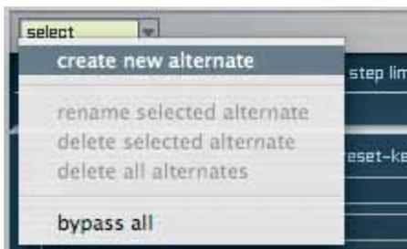
Now enter a name for the Alternate right beside the „select“ pull-down (e.g. Conga Alternate) and confirm with the „Return“ key to instance the new Alternate. As this Alternate is still „empty“ you now have to select the Sections you want to use for this Alternate.
