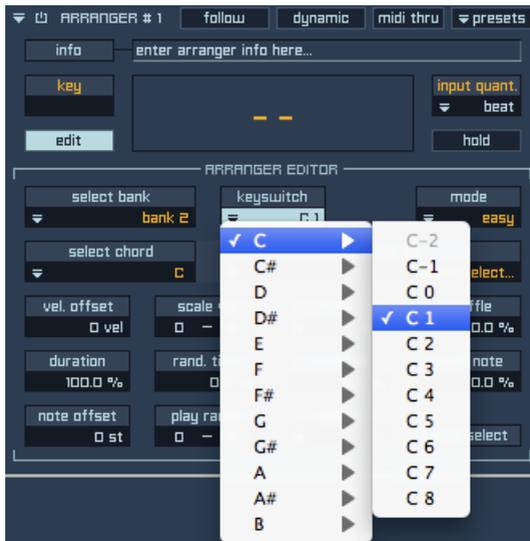
This way each Key Switch note can contain different MIDI files - like 20 Arrangers in one.
