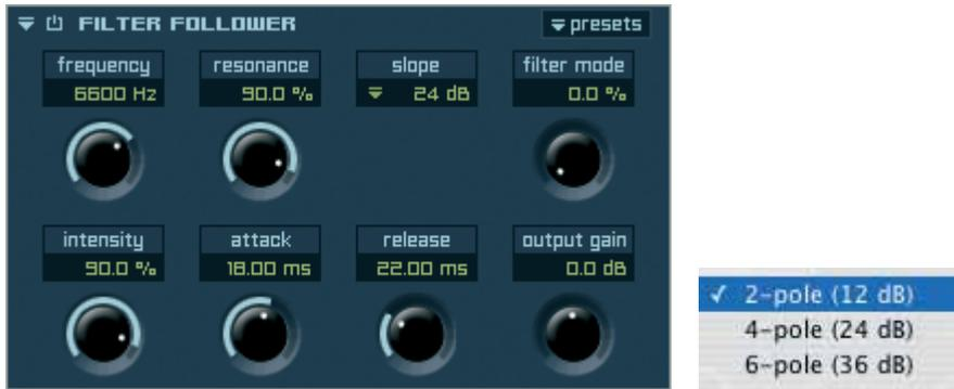
Same as X-Filter. Additionally the Filter Follower changes the settings for „Frequency“ and „Resonance“ of the selected „Slope“ and „Filter Mode“ in a dynamic ratio to the volume of the audio signal.
