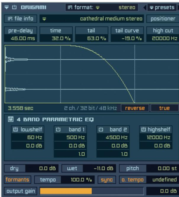
ORIGAMI additionally contains the Élastique SOLOIST Time-Stretch algorithm developed by zplane.development. With this feature you can edit and customize the playback time and tune of your audio and impulse response files. The result is a high-quality manipulation which is specially designed for creating amazing effects.
