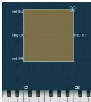
Now you can click and hold with the mouse on this corner and drag/stretch the Zone to the desired size. Using the corners of a Zone you can scale the Zone in the x- and y-axis simultaneously.
