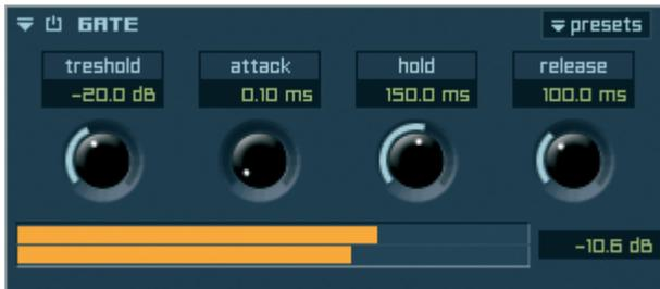
A Gater only lets an audio signal pass through if a determined volume level of the audio signal is exceeded. With the Gater you can avoid noises of the audio signal and also control its dynamic.
