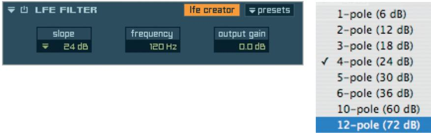
If you are working in a surround format that contains a LFE, you can use this filter to cut high frequencies depending on the selected slope. The “LFE creator” button creates a new additional LFE channel out of all available channels.
