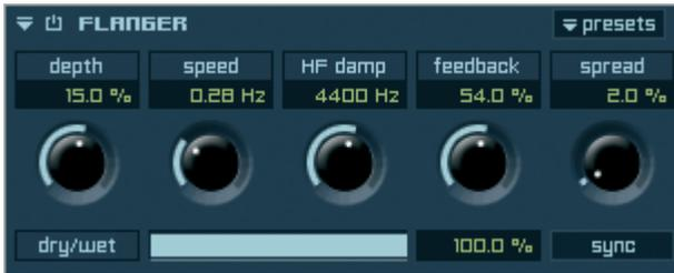
Flanger doubles the audio signal and delays the copy compared to the original signal.
