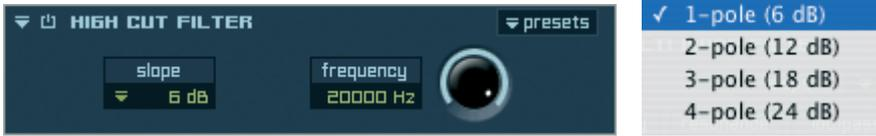
With the High Cut Filter you can cut high frequencies depending on the selected slope.
