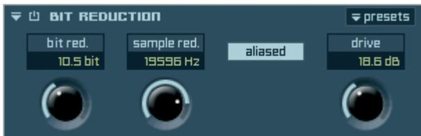
Bit reduction reduces the resolution of the audio signal. Thus you can reduce the sound quality and you can simulate the sounds of older equipment.
