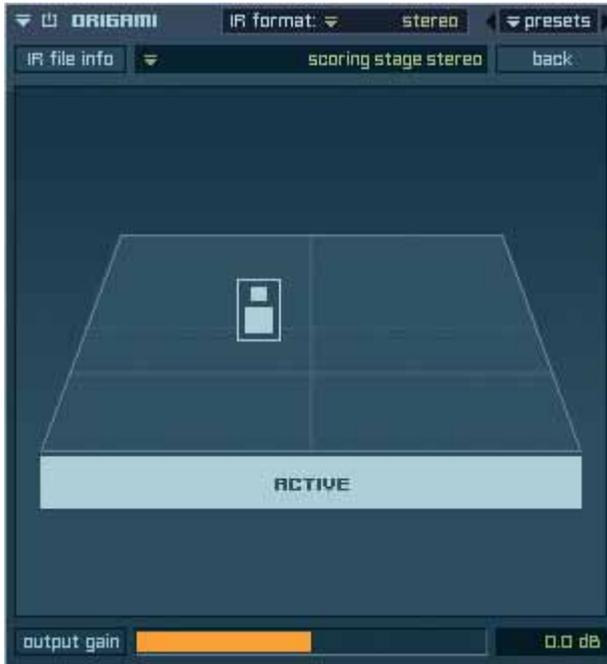
Now you can change the position of the audio signal in your virtual room. To return to the original position of the audio signal in the center, please press and hold the “Alt” key and click on the icon. Now the room position will be reset to its default values.
