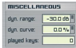
All Notes are mapped to a volume level that is derived from their velocities. This sets the basic volume of a tone. The dynamic range parameter enables you to adjust the dynamic range of the instrument in dB. Additionally you can adjust the dynamic curve of the range limits that you want to use in a session.
