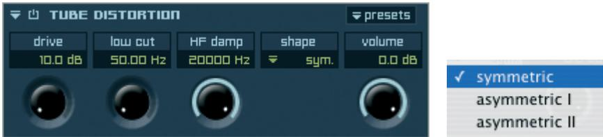
Tube Distortion produces an analog symmetric or asymmetric distortion of the audio signal.
