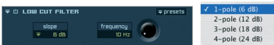
With the Low Cut Filter you can cut low frequencies depending on the selected slope.
