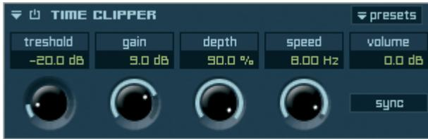
Time Clipper „hacks“ the audio signal and produces an analog rhythmic distortion. This distortion is however not static, but dynamic - in dependence to the „Depth“ and „Speed“ parameters.
