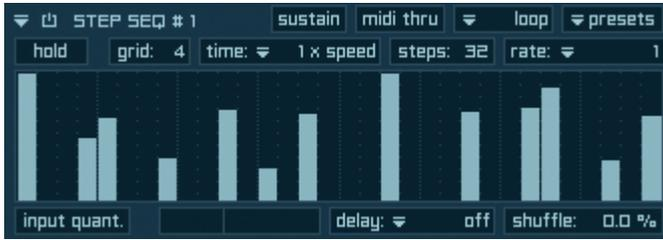
Like the Step Modulator also the Step Sequencer enables you to create a so-called „stepped“ sequences of your instruments. Unlike the Step Modulator (which is commonly used with „pitch“ or „cutoff filter“ as destination), the Step Sequencer only uses the destination “note on” to achieve typically „hashed“ progressions.
