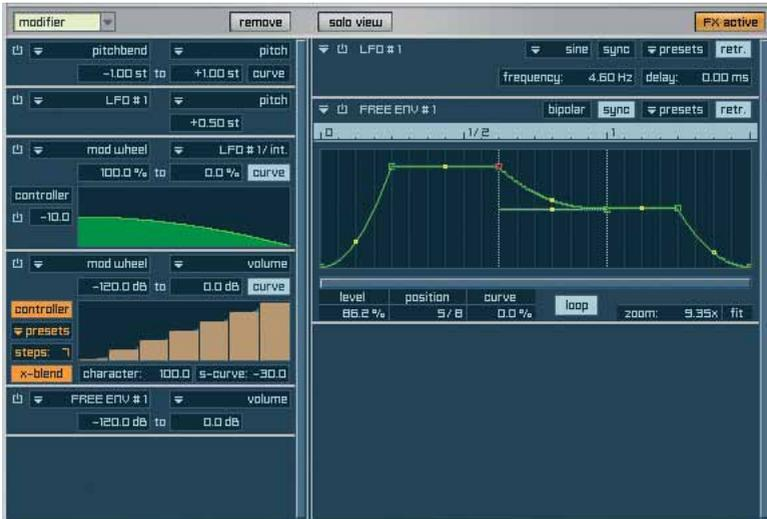
*EXAMPLE: By means of a „LFO“ (internal modulator) as „source“ and „pitch“ as „destination“ you can create a vibrato. Simultaneously you can assign the intensity of the modification, with the „modwheel“ controller as „source“ and the „LFO intensity“ as „destination“, for example. With this combination you will create a typical synth vibrato. If you, however, select „volume“ instead of „pitch“ as destination for the first modifier, you will create a typical tremolo.*
