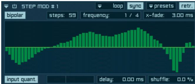
The Step Modulator enables you to create a so-called „stepped“ modulation. In practice this internal Flexible Modifiers is commonly used with „pitch“ or „cutoff filter“ as destination, in order to achieve typically „hashed“ progressions. Independence’s Step Modulator is extended to 128 steps to enable an even more accurate setup. Additionally you can also switch between the „unipolar“ and „bipolar“ view of your settings (see chapter „Free Envelope“).
