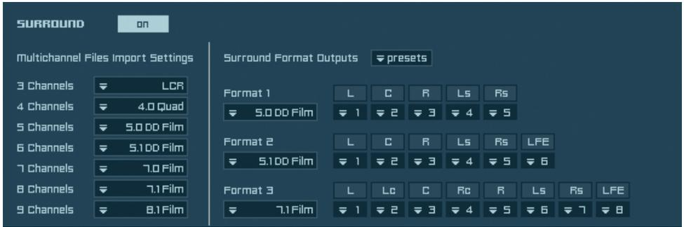
Any surround preference settings get always saved with your Independence Project. If you import multi channel audio files into Independence, you can save your default channel assignment using the appropriate pull-down menus. Additionally you can also save the default settings for three different surround output formats and also create your own presets.
