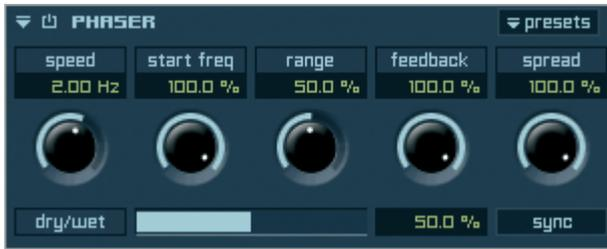
Like „Flanger“ also the „Phaser“ effect splits the input signal, manipulates the frequencies of one split and then sums the two splits back together.
