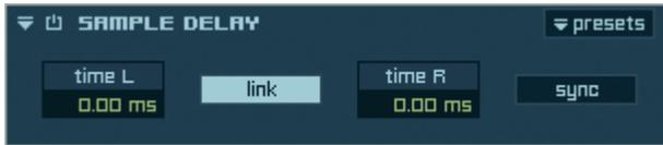
With „Sample Delay“ you can assign a time related movement of the audio signal.
