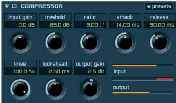
With the „Compressor“ you can reduce the dynamic of your audio signal and thus the differences between soft and loud signals. Thereby you can turn up the overall signal higher without exceeding the available headroom and causing unwanted distortions. The result is more presence and punch of your audio signal.
