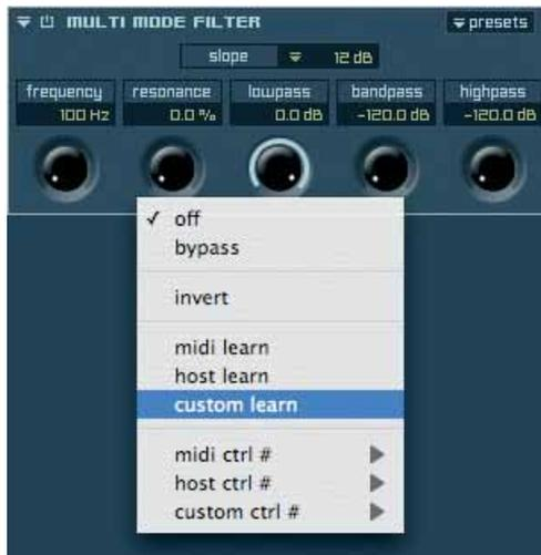
To finish the assignment you only have to click on the knob or button you want to use for the manipulation of the selected parameter. Of course you can also assign any connections manually.
