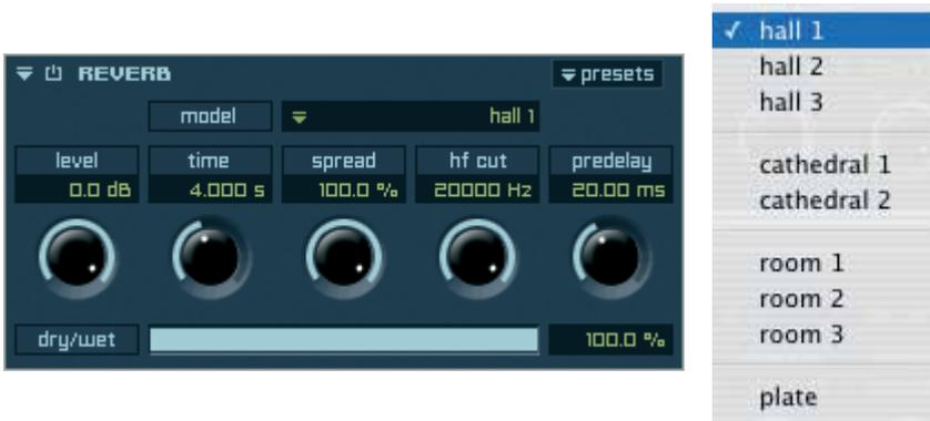
Reverb produces - unlike echo - continuous sonic reflections of the audio signal. Thus allows an extremely real simulation of reverbs of different rooms
