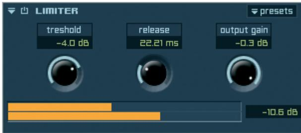
A Limiter regulates the output level of the audio signal gently down, before an over-regulation can take place. Finally the Limiter is also like an „extreme type“ of the compressor, since it works according to the same principle as the compressor, however the level of the compression is substantially higher.
