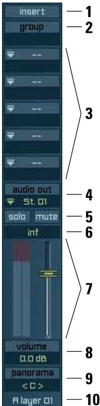
The Layer Channel is a graphic chart of a loaded Layer Patch. As soon as you load a new Layer Patch into Independence, a new channel gets added to the mixer automatically. A Layer Channel contains the following parameters:
