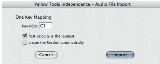
This mapping option is recommended for the import of sounds „key by key“ and enables you to import multiple audio files that are separated by their velocity splits per note - mostly drums or percussive instruments. Thus this mapping option „looks“ at a „velocity“ assignment at the end of the filename, like „02“, „15“, etc.
